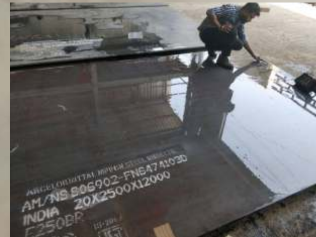
Ultrasonic Testing of plates by Qualified NDT Level-2 Engineer
